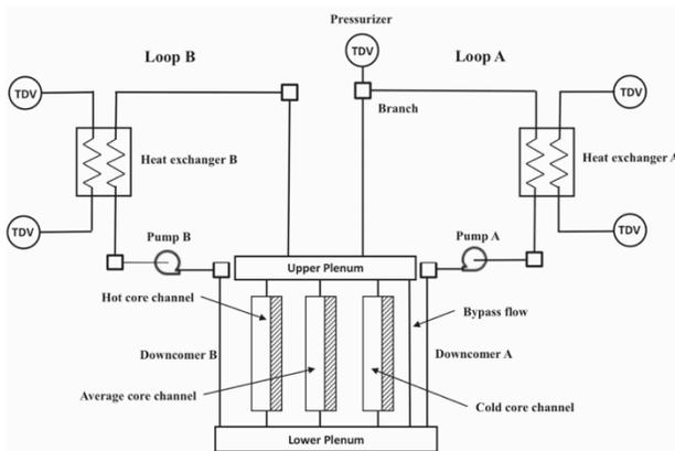
Figure 5 - Scheme of the TMI PWR benchmark.
